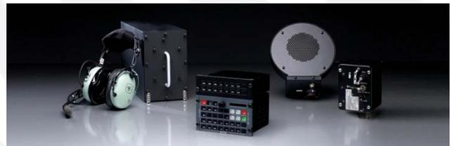
ADAMS is a secure, high-performance communication system, designed to meet the complex requirements of large crew aircraft such as commercial airliners, transport, tanker and mission applications. This modular COTS system supports up to 20 full capability users, 8 intercom only users, 16 radios and 31 receivers, 6 recording outputs, discrete lines and several internal intercom networks.
