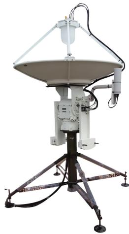
The second antenna, 1.5 meters in diameter, sits atop ORBIT's AL-4012 pedestal mounted on a quad-pod and represents an autonomous tracking system. With its large beam width and high-speed positioner, it is ideally suited for acquisition of fast targets. It can slave the main antenna and can take over the backup or split target tracking during operation. The slaving functionality was built by MORABA and used by ORBIT for tracking.
